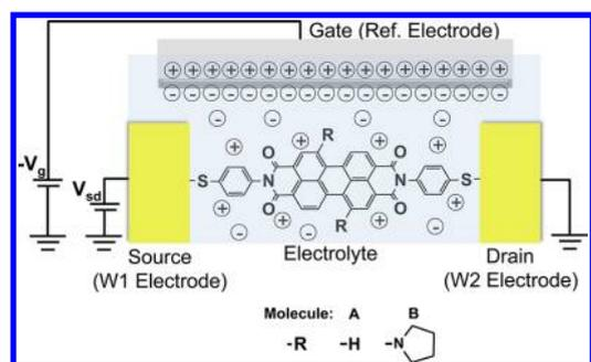
**Figure 1.** Schematic experimental setup of the single-molecule FETs measured in this work. W1 (source) and W2 (drain) electrodes are the Au surface and STM tip electrodes, respectively, in the employed STM configuration. Molecules A and B correspond to the unsubstituted and pyrrolidine-substituted PTCDI blocks, respectively.
