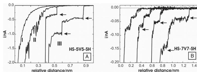
**Figure 2.** (A) Different types of current–distance curves recorded with a gold STM tip, coated with polyethylene, except for the very end of the apex, for HS-5V5-SH on Au(111)-(1 × 1) in 0.05 M KClO<sub>4</sub>, pH ~ 7, at  $E_S = -0.65$  and  $E_{\text{bias}} = 0.10$  V. The setpoint current before disabling the feedback was chosen at  $i_o = 100$  pA. (B) Current–distance ‘stretching’ curves for molecular wires of HS-7V7-SH. Other conditions are identical with (A).
